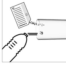
3. Fill the water tank with 0.5 L of fresh drinking water and add 1 Nespresso descaling liquid sachet.
