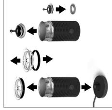
1. Remove the jug from the base, remove seal from lid, remove the whisk, remove the spring from the whisk.
