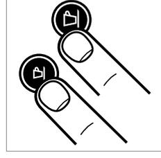
3. Press both the Espresso and Lungo button for 3 seconds.
