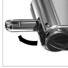
2. Remove the water tank and open the lever.
