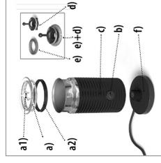
1. Overview: a) Lid, a1) Storage area for frothing spring, a2) Seal, b) Start/stop Button, c) Milk frother, d) Mixer (for hot milk), e) Frothing spring (for milk froth), f) Base.
