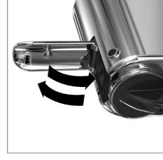
6. Remove the cup. Lift and close the lever to eject the capsule into the used capsule container.
